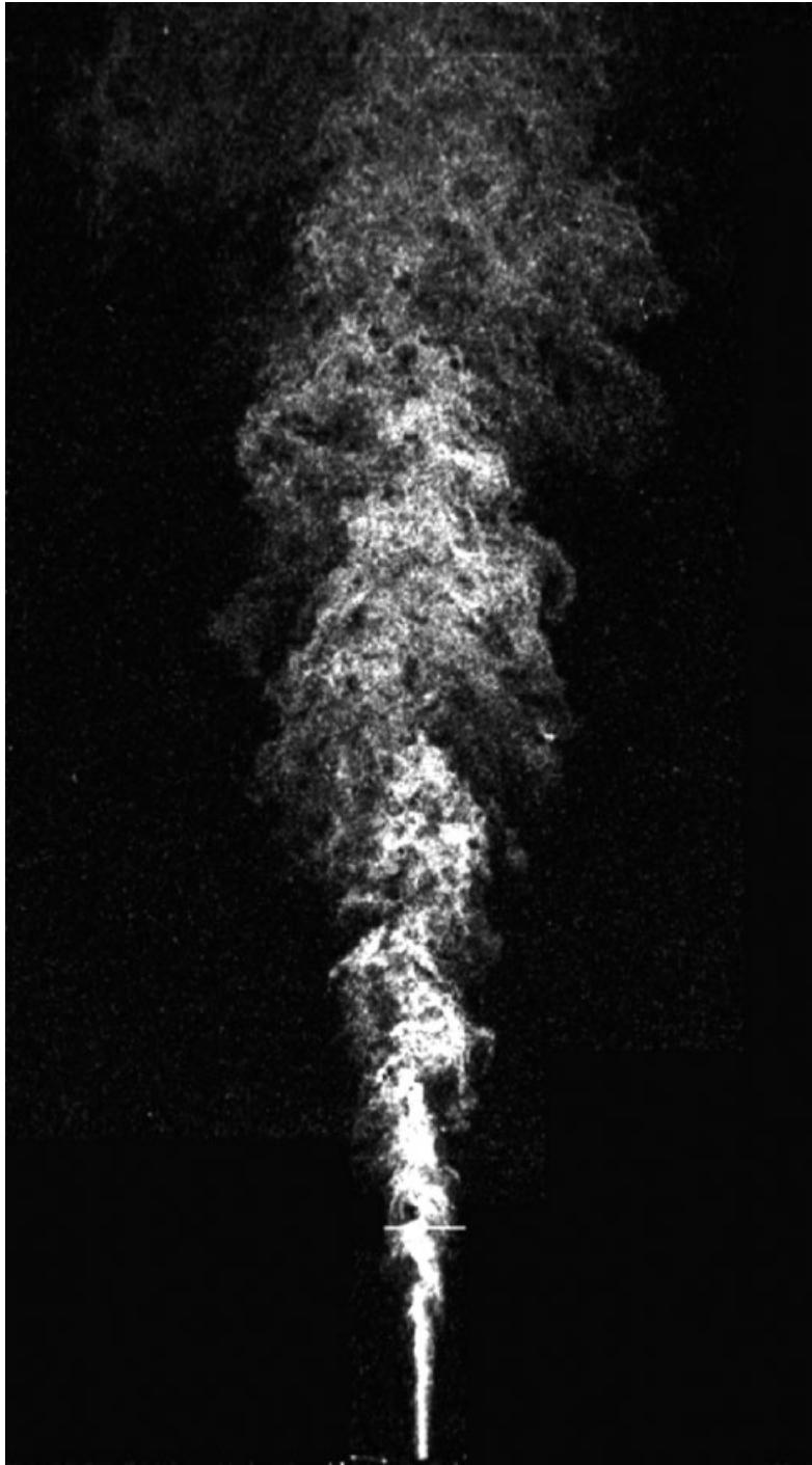
Figure 1. A photograph of a three-dimensional turbulent gas leak jet. The view is of the minor axis and the jet, with a Reynolds number of 33 500, is issuing from an orifice of 40:1 ratio [6, 16, 17].
